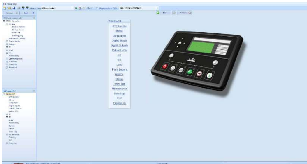
Figure 44 - LSE8600 Controller - Open Scada Information
